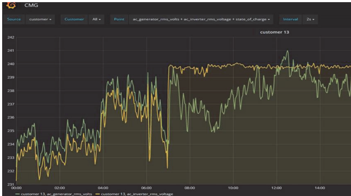
Figure 2: Voltages traces for a single customer within the Mooroolbark Mini Grid trial
