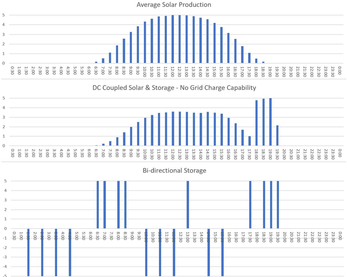
The uni-directional DC-coupled storage helpfully shaves the problematic midday solar generation peak and usefully delivers into the evening demand peak. The result is a more NEM-friendly profile than solar alone. There is only enough storage to serve the evening peak leaving the battery exhausted until its next opportunity to charge during the following daylight hours. This storage cannot charge during the evening eliminating unpredictability.
