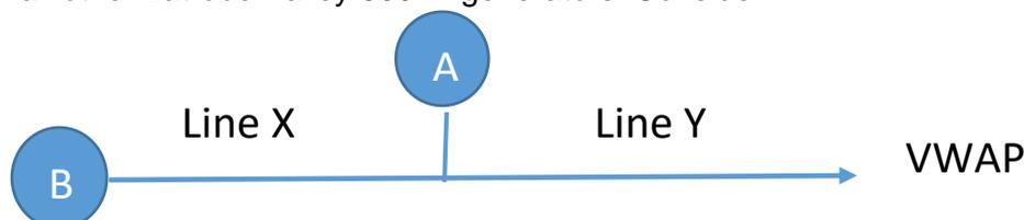
The "hub" approach would see both generators only able to access FTRs from point A, leaving a basis risk for generator B associated with Line X's capacity.
