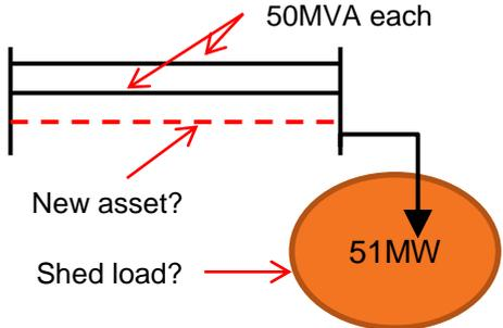
The diagram shows a power supply system. Two parallel horizontal lines represent 50MVA circuits, with a red double-headed arrow above them labeled '50MVA each'. A dashed red line below the top line indicates a potential loss of a circuit. A vertical line descends from the junction of the two 50MVA lines to a circular load labeled '51MW'. A red arrow points to the dashed line with the text 'New asset?'. Another red arrow points to the '51MW' load with the text 'Shed load?'.
