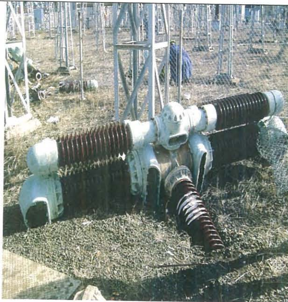
Figure 2 – Failed Circuit Breaker
