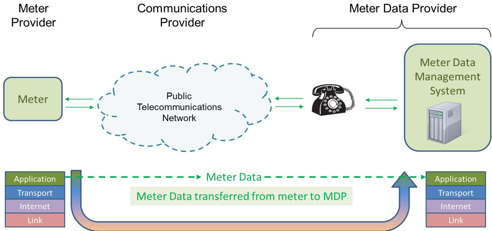
Simplified view of remote meter reading (Type 1 to 4)
