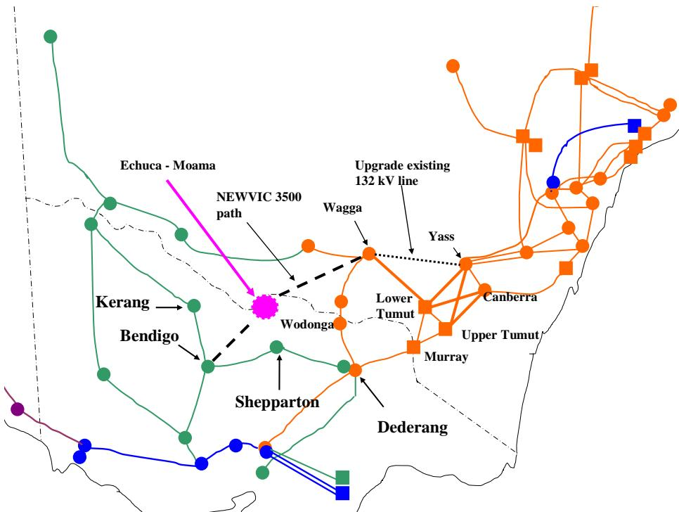
Note. 500kV lines (blue), 330kV lines (orange), 220kV lines (green), 275kV lines (purple),
