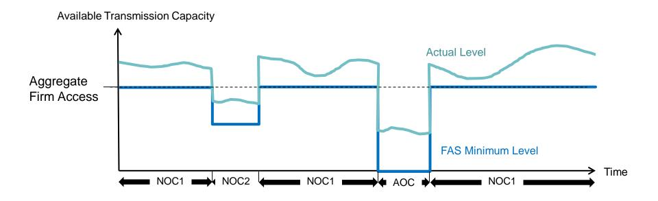
NOC1 = Normal Operating Condition Tier 1 NOC2 = Normal Operating Condition Tier 2 AOC = Abnormal Operating Condition
