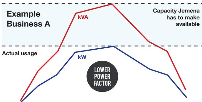
Business A has an inefficient electrical supply. The gap between active power and apparent power is large, meaning the site has a low power factor and a higher than necessary demand charge.
