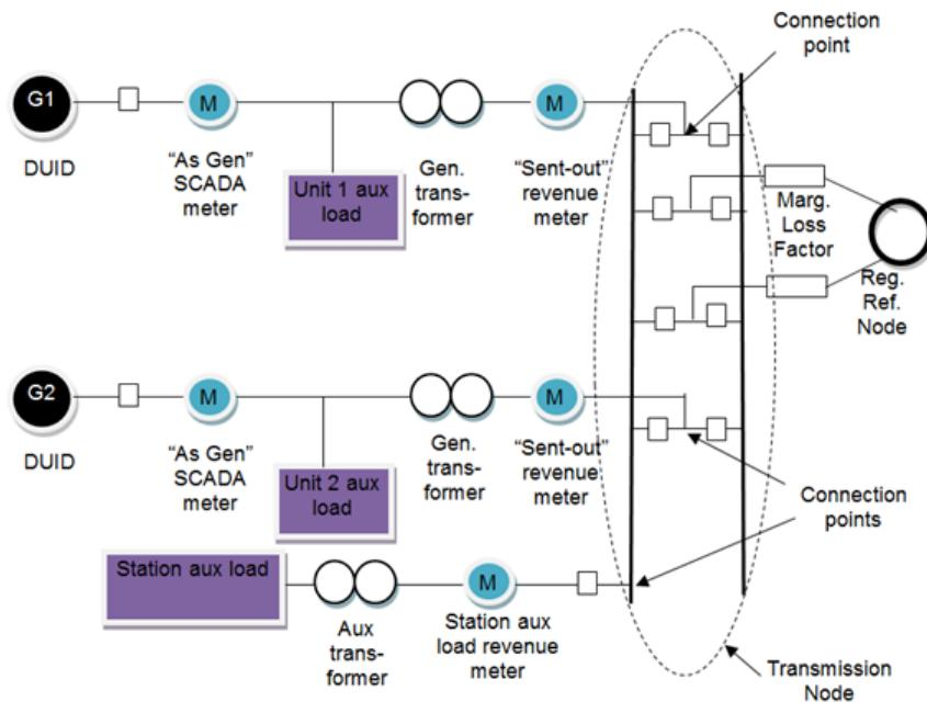
Generating units consume electricity while operating, known as auxiliary load. These auxiliary loads are currently connected in a number of different ways. This includes the load being:
