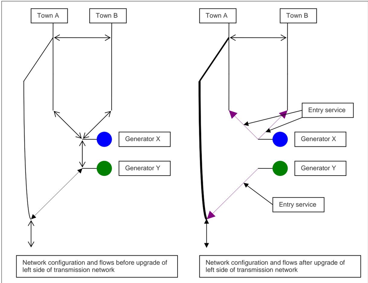
In the above diagram, energy was previously flowing north and south along both transmission lines. The costs for transmission services that Generators X and Y were paying were largely made up of charges for prescribed transmission services.
