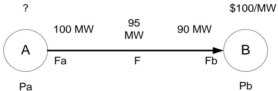
For this example, we assume that there is a flow of 95MW from A to B at the border. There is also 10MW of losses which corresponds to a flow of 100MW at A's regional reference node (Fa) and a flow of 90MW at B's regional reference node (Fb). What value to use as the average loss factor to calculate region A's price (Pa) is not obvious. However, in order to avoid negative settlement residues and keep Pa as high as possible then the following must hold:
