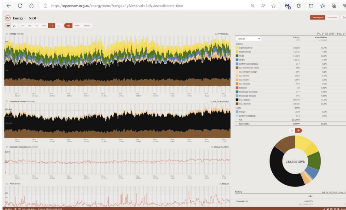
Figure 3b. Screenshot of OpenNEM electricity generation for the same period (a day later) as the data for Figure 3a. This shows that winter solar generation is lower while demand for fossil fuel sourced generation is higher and summer solar generation is higher and total generation is similar to winter.
