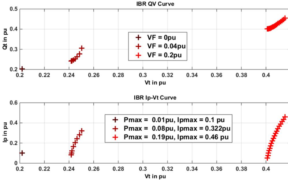
Figure .3 Q-Vt curve and Ip- Vt curve for a severe fault with  $V_F$  of 0.04 pu with 1 pu reactive current injection as a function of active current injection **for different retained voltages at PCC**
