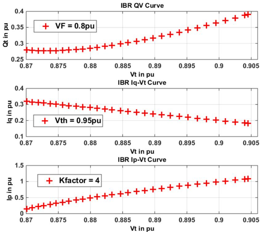
Figure .5 Q-Vt curve and Ip & Iq- Vt curve for a shallow fault with VF of 0.8 pu with Kfactor of 4 and Vth of 0.95 pu for reactive current injection as a function of active power injection
