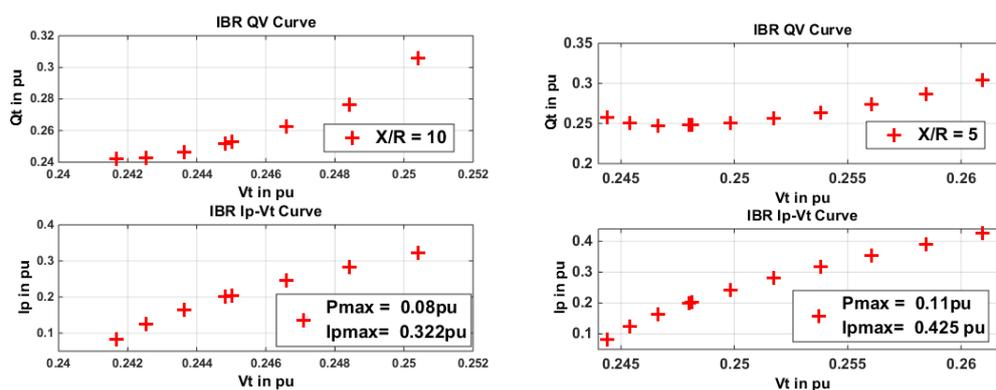
Figure .2 Q-Vt curve and Ip- Vt curve for a severe fault with  $V_F$  of 0.04 pu with 1 pu reactive current injection as a function of active current injection **for different X/R ratios**
