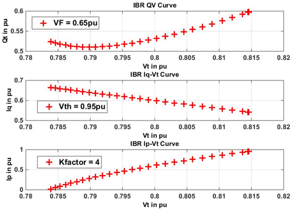
Figure .4 Q-Vt curve and Ip & Iq- Vt curve for a shallow fault with VF of 0.65 pu with Kfactor of 4 and Vth of 0.95 pu for reactive current injection as a function of active power injection
