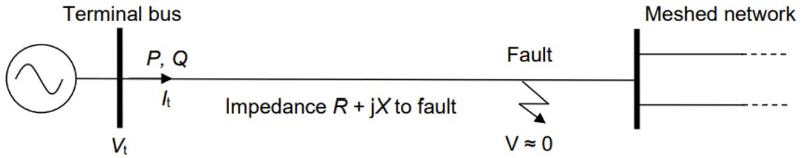
Figure 1 Hard short circuit located radially with respect to a generator.
