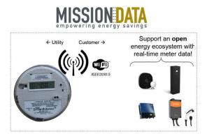
IEEE 2030.5 supports any internet capable link. The above figure suggests the utility meter support the now universally supported Home Area Networking standard 'WiFi' (as described in the IEEE 802.11 series of standards).
