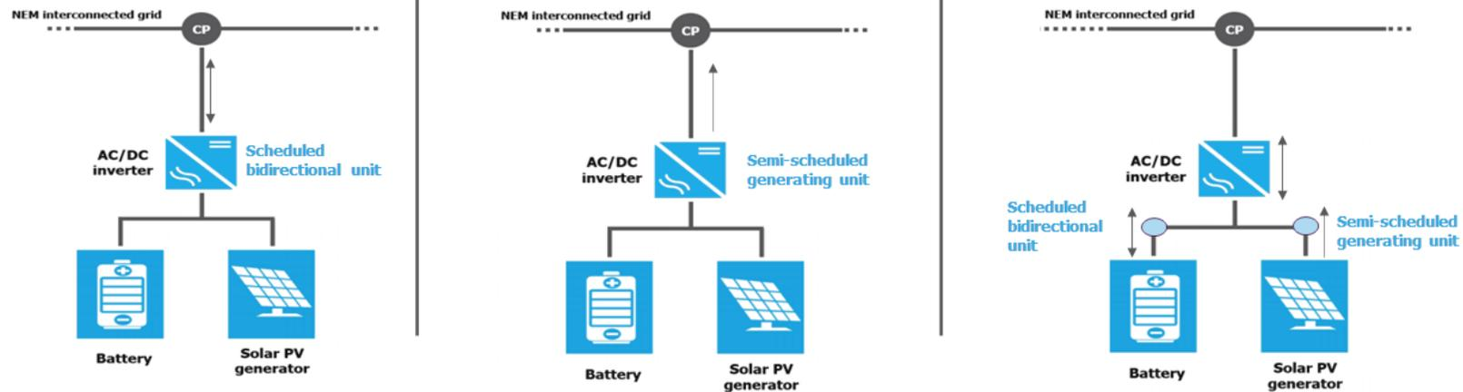
This diagram is an example of a stand alone DC coupled system. These options could also be used in a hybrid facility. A DC coupled system could vary in the number and type of plant behind the inverter.
