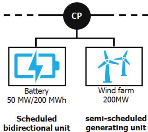
In the mode where **only the battery** is in service, the performance will be assessed against the requirements for a scheduled bidirectional unit. That is, AEMO would only consider the requirements for the battery at the point of obligation.
