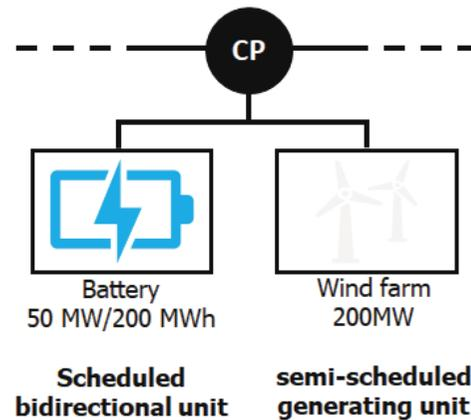
In the mode where **only the wind farm** is in service, the performance will be assessed against the requirements for a semi-scheduled unit. That is, AEMO would only consider the requirements for the wind farm at the point of obligation.
