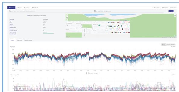
AusNet Services Explore dashboard that provides operational teams and network engineers visibility of near real-time individual customer and aggregated power quality data
