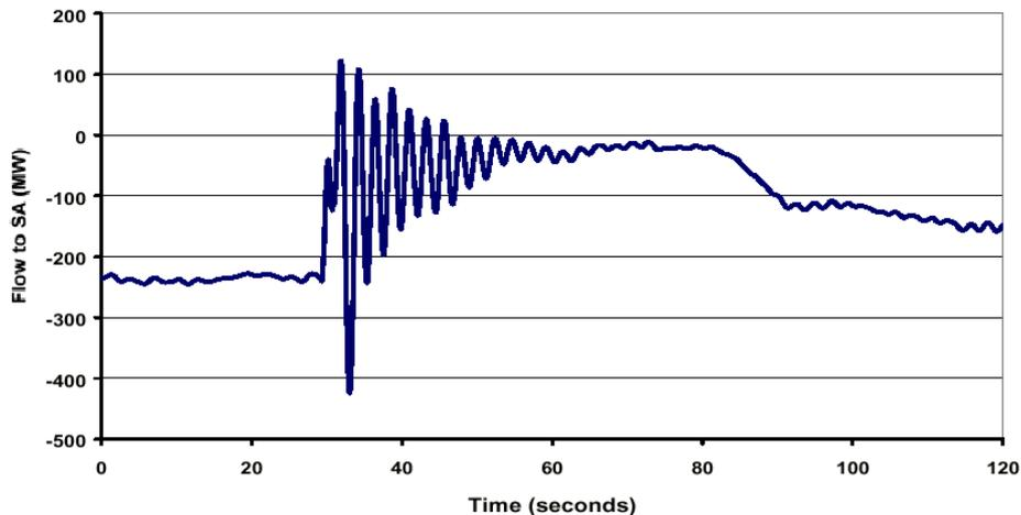
This type of response is required it shows a dynamic active power response from all units in the system. The settling is caused by the rotating masses settling into a new steady state equilibrium. The rules expect this type of response and the technical standards require the system to have a 5 second halving time. Without dynamic active power present in the power system in all areas, the system will suffer greater load shedding, and more severe power system disruptions.
