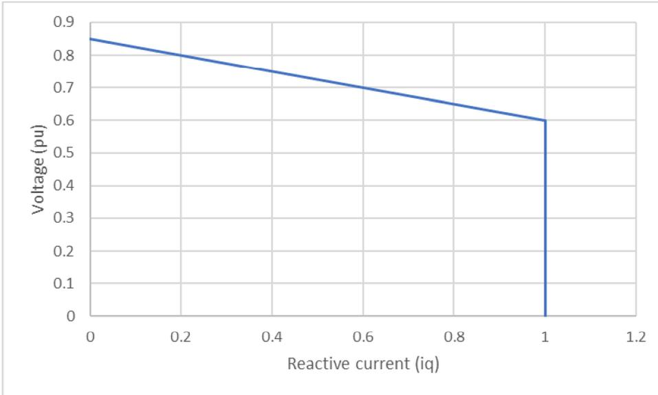
Figure 2 - X/R =3 site, diQdv settings under new proposed wording. Settings points: [0.85, 0], [0.6128,0.9487], [0, 0.9487]
